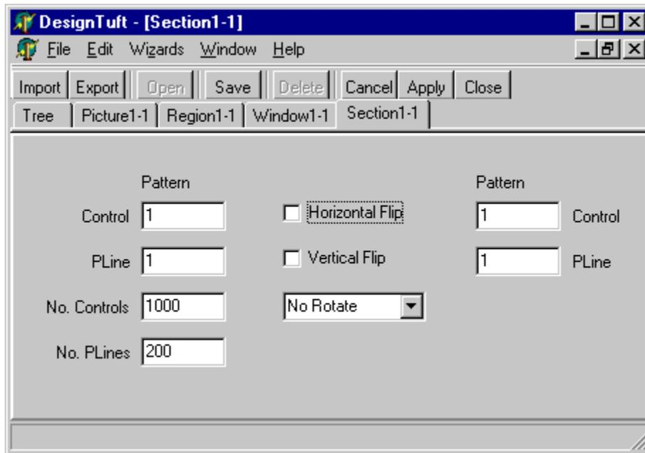
The originating point is the pattern control and pline (pattern line) defined on the left. The destination point is the pattern control and pline defined on the right. The width of the rectangle copied is the number of controls specified; the height of the rectangle copied is the number of plines specified.
