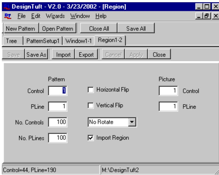
The originating point is the pattern control and pline (pattern line) defined. The destination point is the picture control and pline defined. The width of the rectangle copied is the number of controls specified; the height of the rectangle copied is the number of plines specified.
