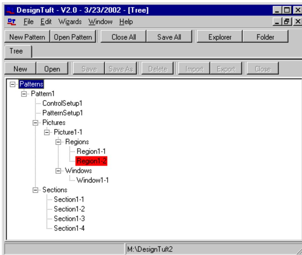
When the Tree tab is selected a hierarchical view of currently opened patterns is displayed. Each item or node in the tree view is referred to as an object. The root of the tree is the Patterns object which contains a list of all open patterns.
