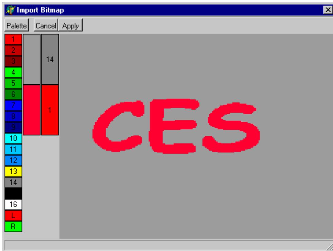
After clicking the Import button, a image of the bitmap is displayed. On the left, three columns of color information appear. The first column is the palette which is used to select colors. The second column contains the colors that occur in the imported bitmap. The third column is used to assign palette entries to bitmap colors.
