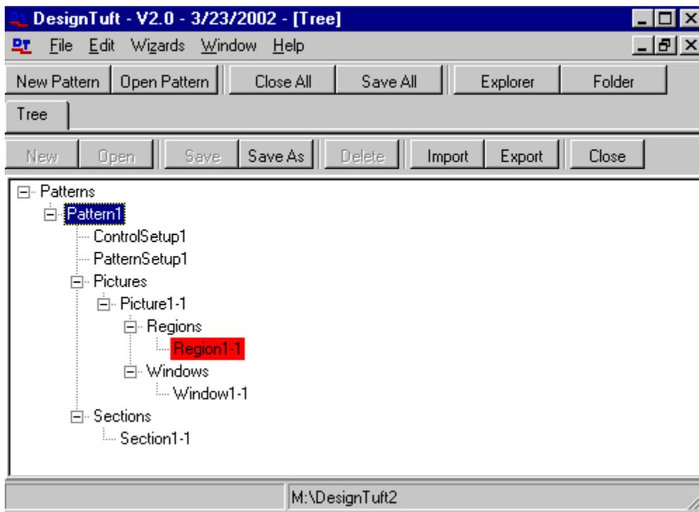
To create a TUF pattern in DesignTuft, select the pattern name in the Tree view screen and then left click the Export button in the toolbar. Note that a pattern diskette can contain one or more TUF and DAT files.
